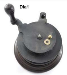
**1.** Remove the brass cap nut on the front of the winch, as shown in Dia 1, using a 10mm spanner
