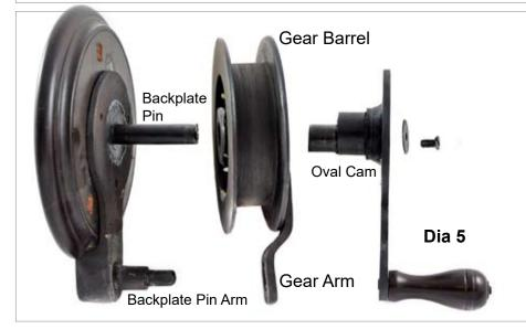
**5.** Now place the gear barrel over the pin from the back board. Reassemble the winch component parts as shown in Dia 5. The last part on the right with the winch handle has an oval cam on it, ensure this is located correctly in the central gear system. It will lock back fully home into position. Also make sure the gear arm locates back over the back plate pin arm.
