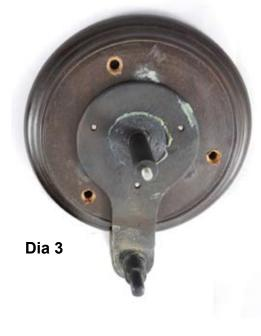
**3.** Screw the wooden back board into position on your wall using the screws provided and the 3 holes in the board itself. Screw it to the wall with the location arm at the bottom as shown in Dia 3 **Dia 4.** Back of gear barrel with rope fitted. The gear inside is loose and will come out. Just place it back into position if it does
