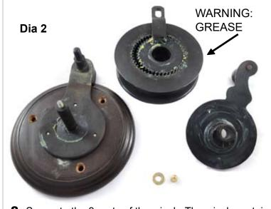
**2.** Separate the 3 parts of the winch. The winch contains a lot of grease so please be careful not to get any on your clothes.
